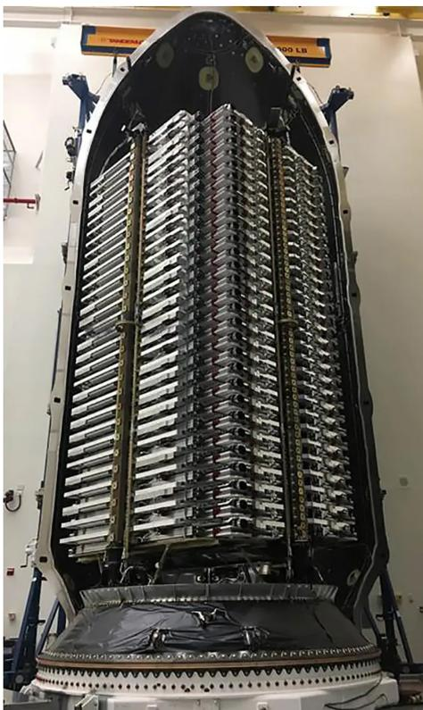
A SpaceX rocket payload can release more than 50 Starlink LEO satellites in one launch. After entering orbit, each satellite migrate to its proper place in the constellation.
