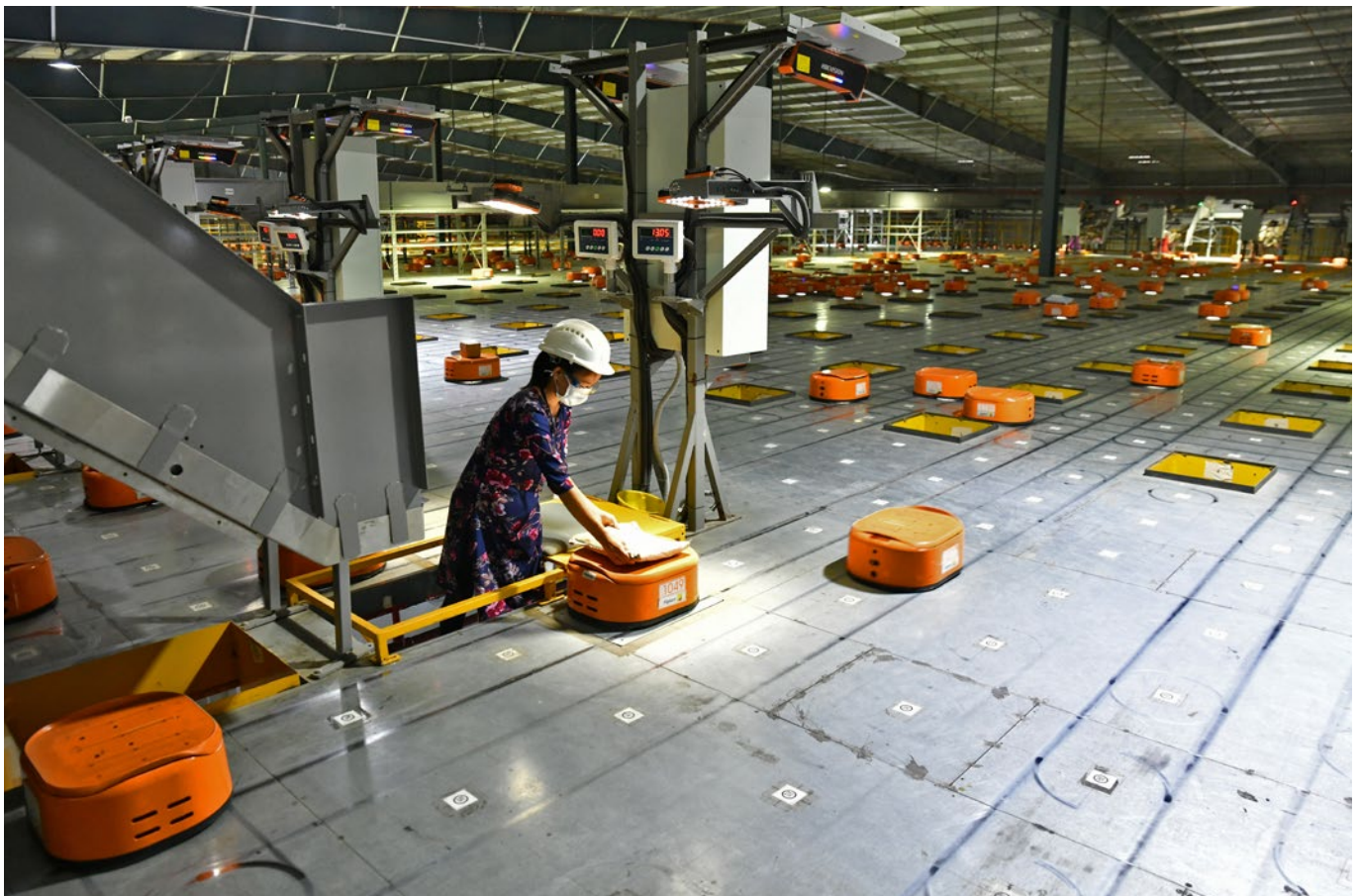
A worker uses automated guided vehicles at Flipkart, a leading e-commerce firm in India, to sort items inside its fulfilment centre (Bengaluru, 2021).
